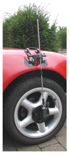
The **Clamps** main property is its high holding force. It allows attachment of heavy equipment securely to the wheel nuts, even on extremely bad roads.
