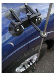
Holding Plate with 4 Suction Cups and lengthened Slip Joint
